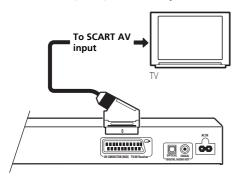
Use a SCART cable (not supplied) to connect the AV CONNECTOR (RGB) TV/ AV Receiver output to a SCART AV input on your TV (or AV receiver).
